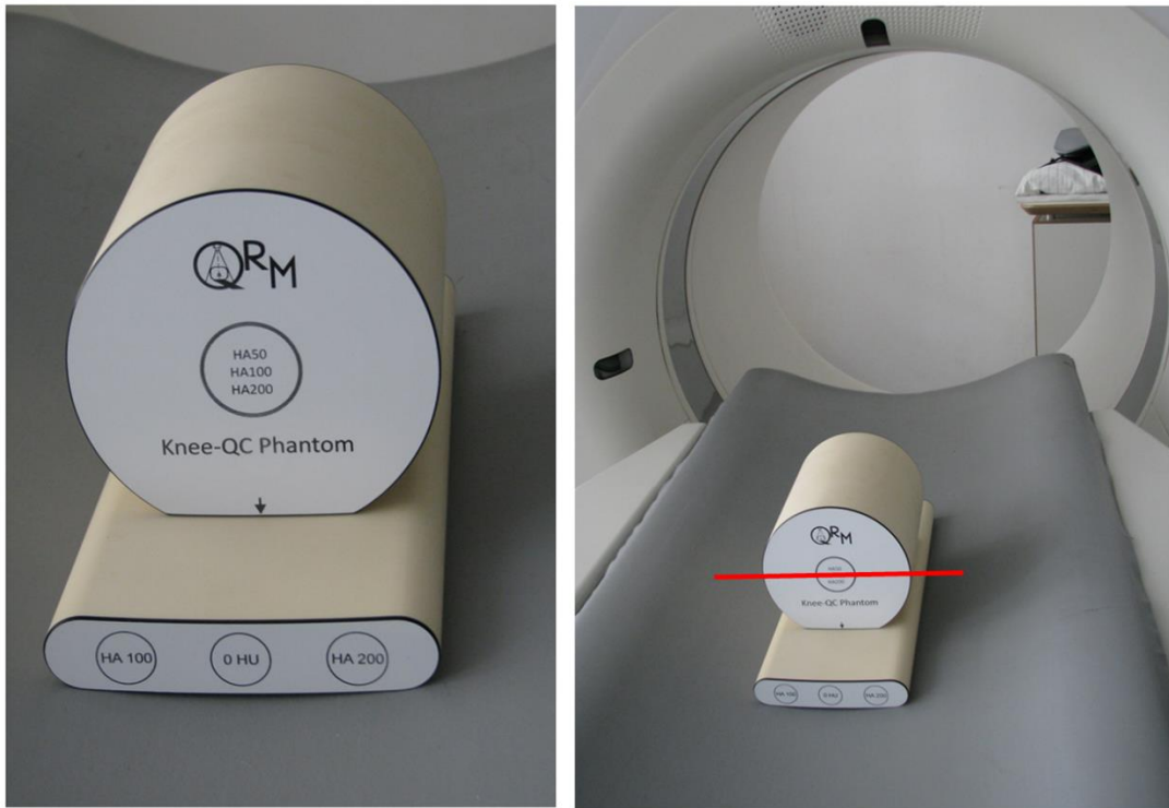
Fig. 4-2: Left: QRM™ Knee QC phantom and BDC, Right: setup in CT scanner; the red line indicates how the knee phantom should be positioned in the gantry to determine the table height
